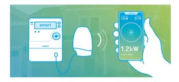
Powerpal will connect to your smart phone automatically whenever it is within Bluetooth range of your electricity meter – this is typically between 50m and 100m depending on the construction of your home
